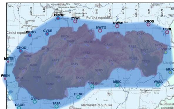
**Fig.4** Distribution of foreign permanent stations with potential for incorporation into SKPOS solution
