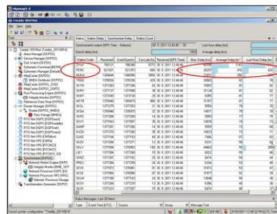
**Fig.8** Bigger foreign permanent stations incoming data delays monitored by service control software.
